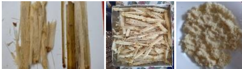
Figure 4. Show The Results Of Fiber, Skin, And Powder Separation
