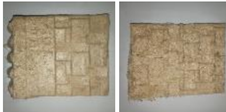
Figure 12. Showing the result of finishing with wood glue and polyurethane
