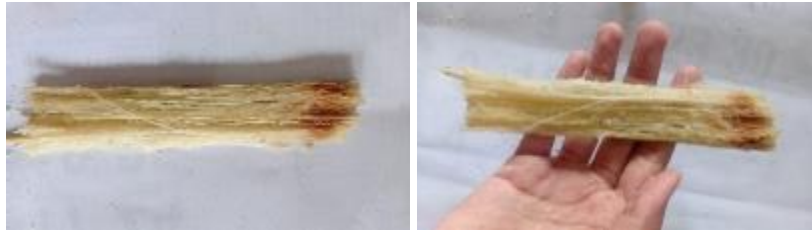
Figure 3. Shows The Appearance Before And After The Softening Process Using Hot Water With Salt And Liquid Soap
