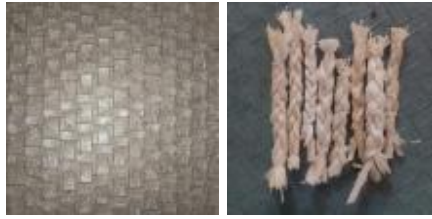
Figure 11. Showing The Result Of Forming A Powder Pattern Pressed With Wood Glue And Fibers Woven Into A Braid
